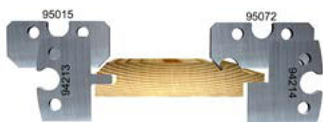
Large tongued, grooved and beaded timber
