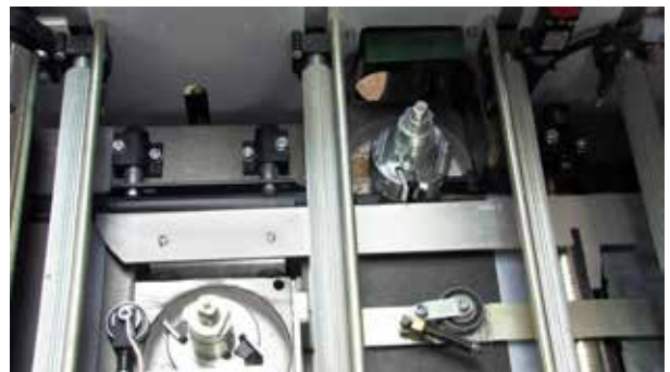
Installation jig for adjusting fences.
