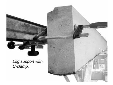
**Tip:** if the log is crooked the long-groove will not be milled in the centre. To centre the long-groove milling, set two Versatile Log Fences (art. no. 4510-720-6104) at the same distance from the guide rail as the non-adjustable log fences on the Logosol Sawmill. Fit C-clamps over the log and and the versatile log fences at the log ends. This will also give a smoother surface.
