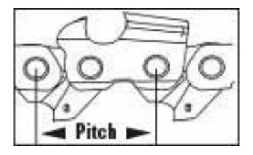
Distance between three rivets divided by two as shown.
